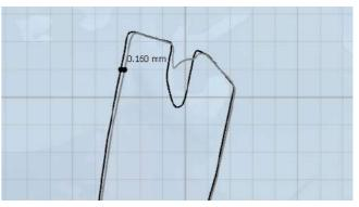
The next thing we were able to do was to utilise the 3Shape software to take sagittal and transverse cross sections at varying points of the meshed scans to obtain quantitive data on the accuracy of the prints. Fig. 5 & 6 show an inaccuracy of 0.15mm or 150 microns which was not accurate enough in our opinion.
